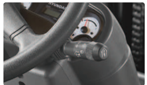
Multi-function switch lever
