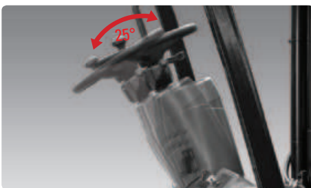
Adjustable steering wheel
