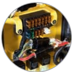
Concentrated Fuse Box for Easy Inspection
