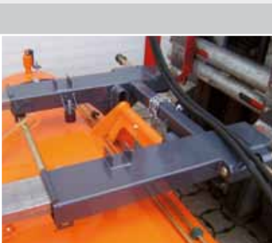
Hitch system with 3D levelling (standard)
