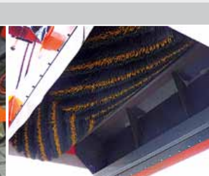
Special V-brush for sticky and fine dirt
