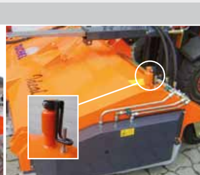
Brush adjusting lever facilitates brush adjustment
