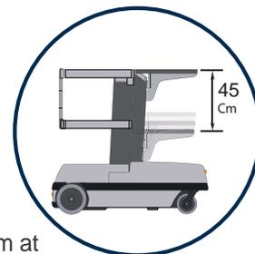
Loading platform at maximum height corresponds to the mast. It is very easy to place even heavy packs, using the column as the setting base and letting it slide up to the material tray.
