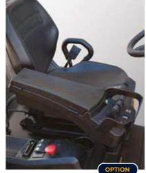
Fingertip control lever and adjustable armrests The electric control lever makes operation almost effortless. The ergonomically designed armrests can be adjusted up and down and from front to back, to fit different body shapes and reduce fatigue.
