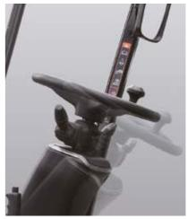
Adjustable steering column The steering column can be adjusted to the operator's preferred position using a single lever.
