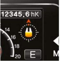
**Speed adaptive steering** The steering angle sensor displays the machine's travel direction on the screen. The speed of the truck is reduced as the steering angle increases.
