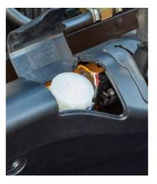
Brake oil reservoir with level sensor The enhanced brake oil reservoir, located in the upper left dash, is equipped with an electronic level sensor that alerts the operator with an audible alarm when the level is low.
