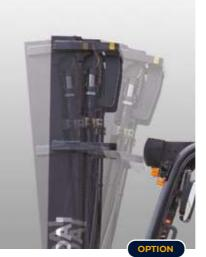
Auto fork levelling system This feature ensures that mast tilting stops smoothly when the forks are in a level position, improving both productivity and safety.
