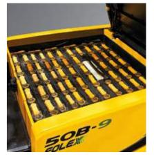
**Easy battery maintenance** The battery cover opens fully to improve access. It is equipped with locking gas springs for safe and easy maintenance.
